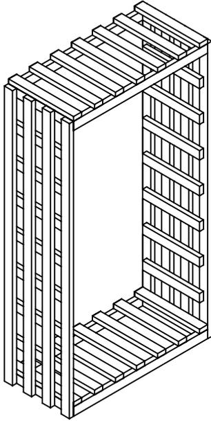
2. Nail only the bottom shelf to the side rail. Leave the top shelf to keep the spacing.
